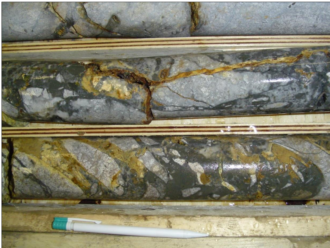
Figure 4: Strongly silicified rhyolite tuff, brecciated, with dark chalcedony and stibnite stockwork infill plus limonite (orange) after sulfides (KG-BL-1: 104.1-105.5m; 2.98g/t Au)
