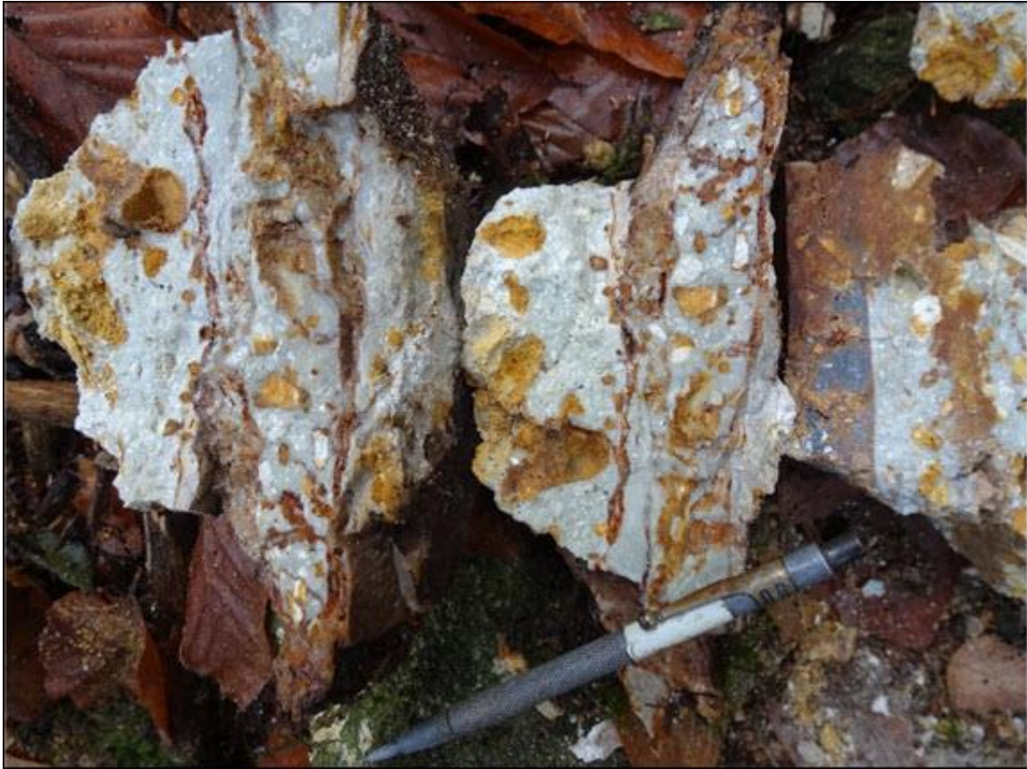
Figure 5. Hydrothermally altered rhyolite pyroclastic rock from the area of the exposed cryptodome including a chalcedonic veinlet with finely disseminated marcasite in the far-right piece (above scribe end), 506g/t As, 107g/t Sb.
