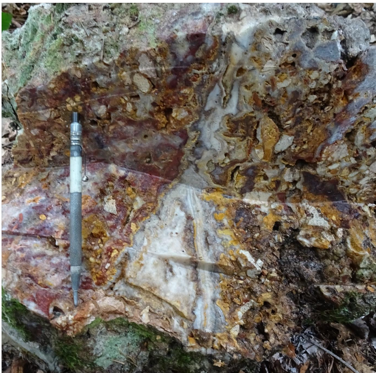
Figure 3. Slabbed surface rock specimen (Sample 95979, 613m RL) displaying a crustiform-colloform banded chalcadonic quartz vein cross-cutting strongly brecciated and silicified rhyolite. This texture records episodic deformation events within the upper level of the epithermal system. This brecciated quartz assemblage returned elevated pathfinder values of 158ppm As , 156ppm Sb and 0.74ppm Tl (with gold and silver below detection limits).
