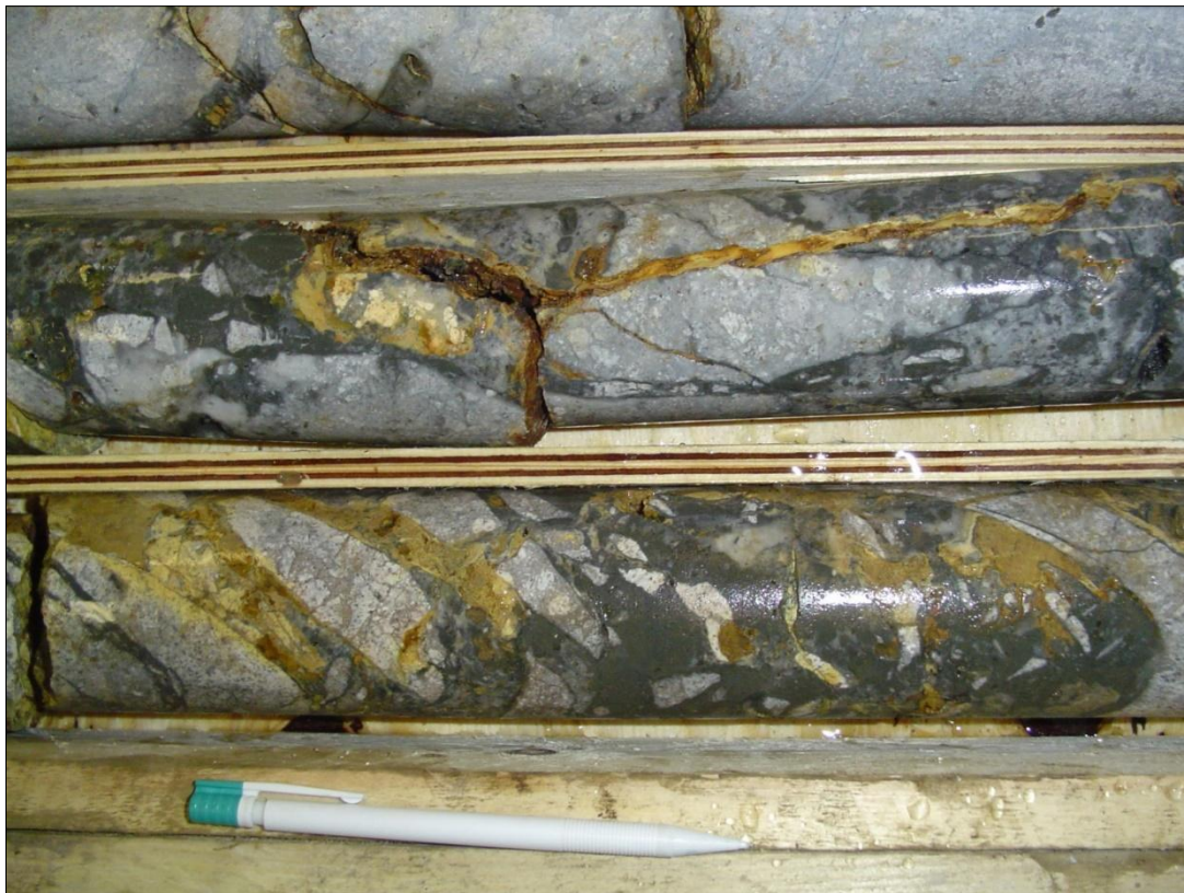
Figure 1. Strongly silicified rhyolite tuff, brecciated, with dark chalcedony and stibnite stockwork infill plus limonite (orange) after sulfides ( 2.98g/t Au & 19.5g/t Ag ; 104.1-105.5m; KG-BL-1).
