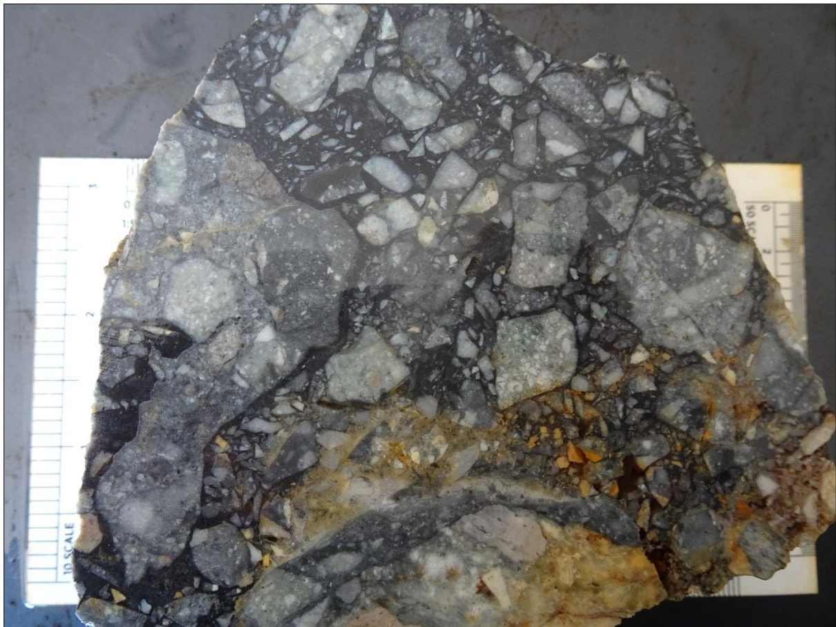
Figure 2. Slabbed rock sample 95990 (421mRL) displaying a diagnostic hydrothermal breccia texture. The sample shows distinct quartz vein fragments - ranging from low-temperature chalcedonic quartz to higher-temperature vein quartz - set within a polymict quartz vein, pyrite-rich matrix from the southern portion of the BL Vein trend. This brecciated epithermal assemblage returned assays of 0.18g/t Au, 2.6g/t Ag, 644ppm As, 1,104ppm Sb and 4.6ppm Tl .
